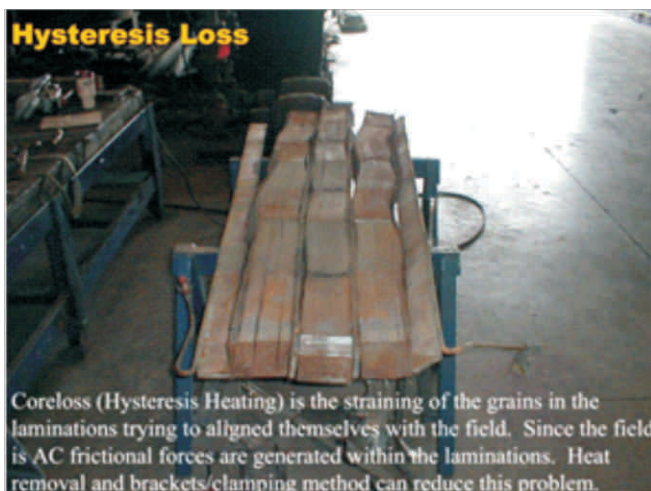
Figure N represents shunts and yokes that have not been maintained properly
