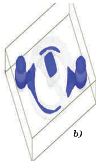
Fig.5 Solidification for gating ratio of 1:2:2, with a) temperature distribution and b) liquid fraction.
