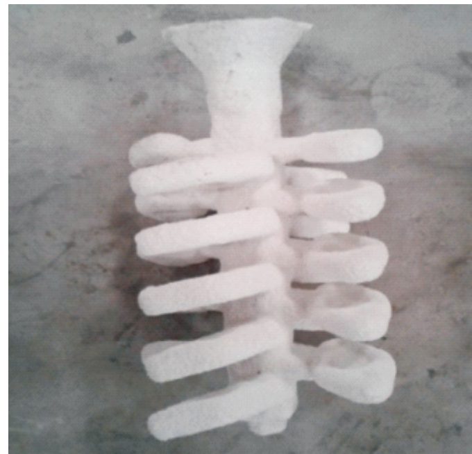
Fig. 2 : De-waxed tree (Ready for pouring)
