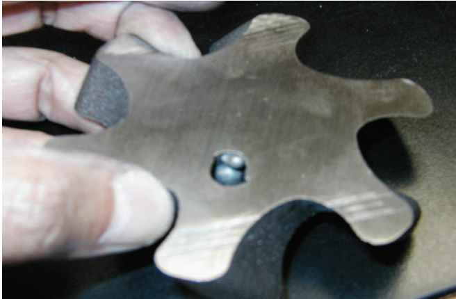
Figure 6. Exudation of semisolid metal into a void in the center of a casting
